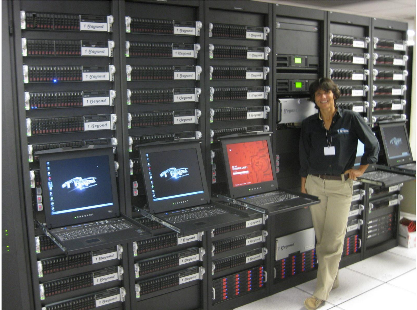
Rony Sebok with the Installed 1 Beyond DDR systems. Points of interest: Main DDR Systems include: 6 Racks: 44 DDRs, 10 Players, 144TBs EzHDSAN Shared Storage and 2 LTO5 LTFS 24 tape Robotic Libraries.
